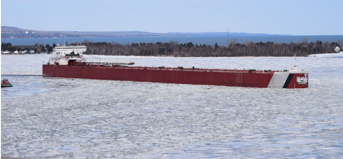
Photo II-1: 1000' M/V Edwin Gott in brash ice transiting the Twin Ports' Superior channel (Daniel Rust)
